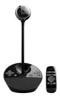
Group add-on solutions include microphone(s) and speaker(s) optimized for group situations that are used <u>in place of</u> the BYOD device's integrated mics and speakers. Note that some add-ons also include a video camera, and as a result provide both enhanced (group ready) audio and video functionality.
