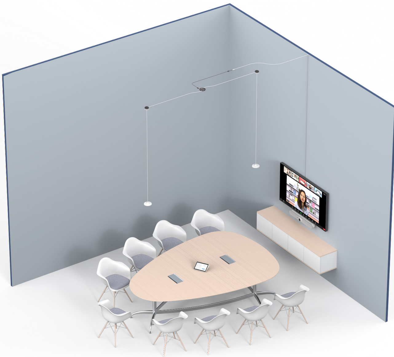
Figure 2 - Two Mic Pods with Pendant Mounts. Both Mic Pods are connected to a Mic Pod Hub, and the Mic Pod Hub is connected by a Rally Mic Pod Extension Cable. Mic Pods are spaced 2.4 meters (8 feet) apart, with the Mic Pod Hub in the middle to maximize cable usage. Note: Image not to scale.
