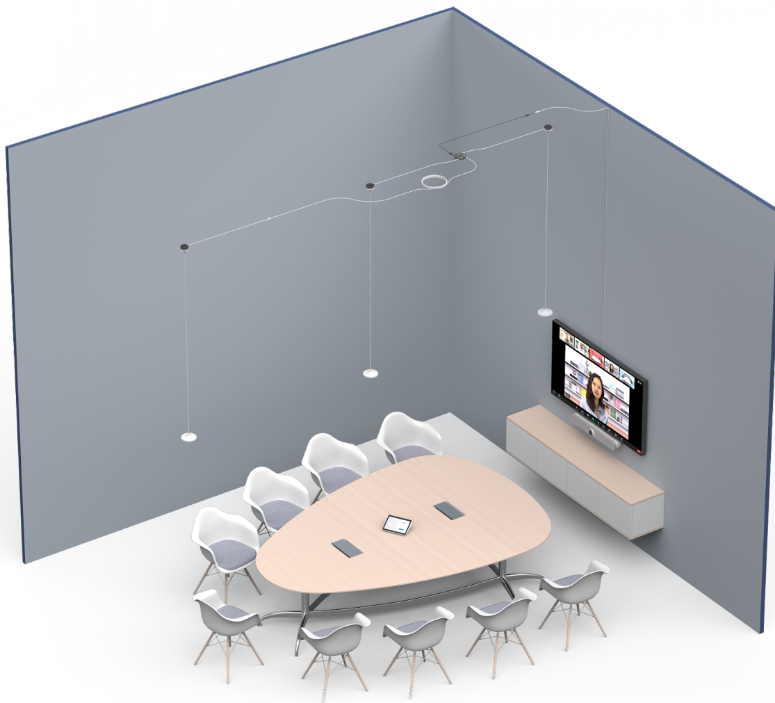
Figure 3 - Three Mic Pods with Pendant Mounts. The first two Mic Pods are connected to a Mic Pod Hub, and the Mic Pod Hub is connected by a Rally Mic Pod Extension Cable to a Rally Bar/Rally Bar Mini system. The third Mic Pod is connected to the Mic Pod Hub with an Extension Cable. Mic Pods are spaced 2.4 meters (8 feet) apart, with the Mic Pod Hub in the middle of the first two Mic Pods to maximize cable usage. Note: Image not to scale.
